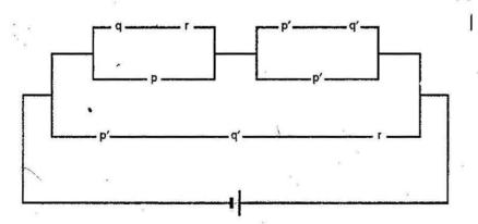
Use the laws of Boolean algebra to simplify the circuit. Construct the network for the simplified circuit.
