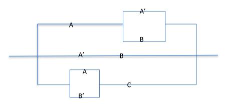
A,B and C represent switches in 'on' position and A', B' and C' represent them in 'off' position. Using Boolean algebra, simplify the function and construct an equivalent switching circuit.
